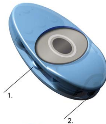
Figure 2. Front view 1. lights-indicators 2. control button
