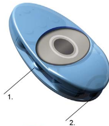
Figure 2. Front view 1. lights-indicators 2. control button
